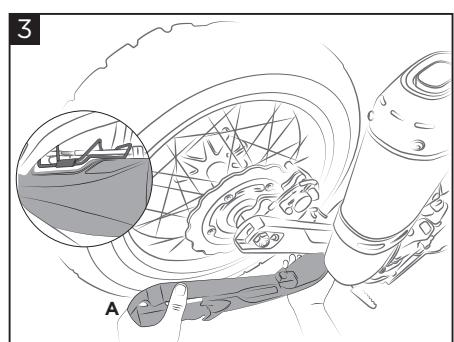
**Mount the fork protection (A) framing it with the support (C) and tighten the zip ties (E).**
