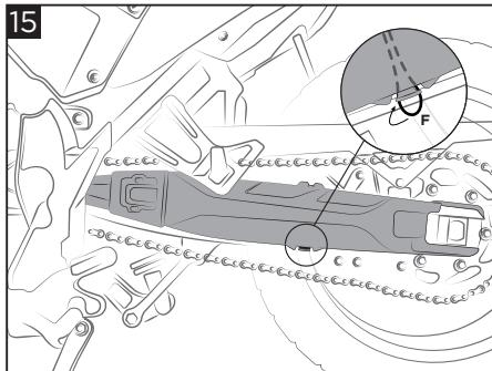
**Mount the fork protection (B) framing it with the support (D) and hook the rubber band (F).**
