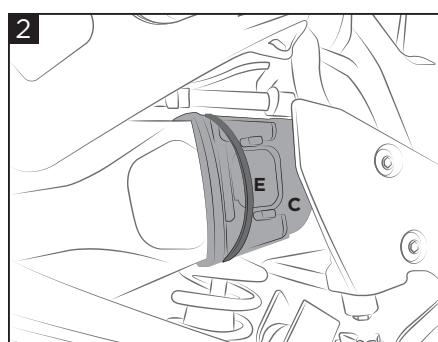
**Place the support (C) and close the zip ties (E) without tightening.**
