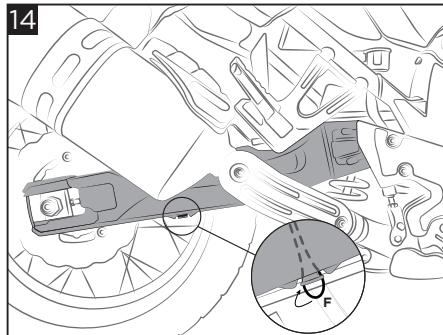
**Mount the fork protection (A) framing it with the support (C) and hook the rubber band (F).**
