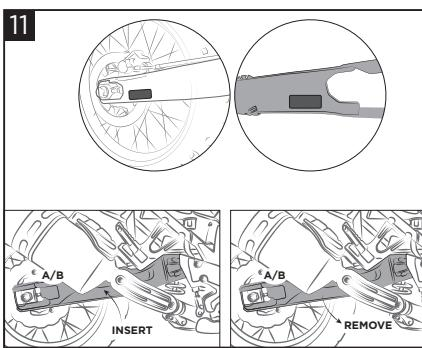
**Place the swingarm protections (A)/(B) and applying pressure in the fixing areas of the velcro and remove it, checking that the velcros are placed correctly on the protection and the swingarm.**
