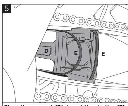
**Place the support (D), insert the zip ties (E) as shown in figure and close them without tightening.**
