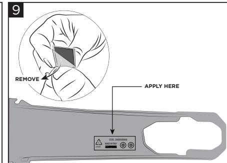
**Clean perfectly the swingarm and the teket magnet protection removing any trace of dirt, grease and oils in the indicated area. Remove the biadhesive's protective film (H) from one side and paste it on the inside of the protection (A)/(B), as shown in figure (above the plastic details panel).**
