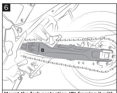
**Mount the fork protection (B) framing it with the support (D) and tighten the zip ties (E).**
